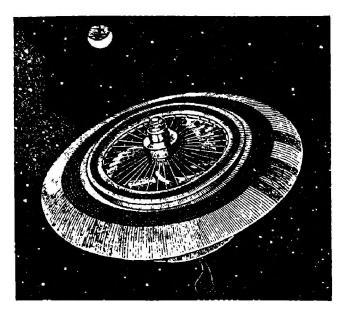
The great hubbed wheel which Capt. Noordung conceived as the proper design for an Earth satellite in 1928, has remained the basic model for all those which followed. A solar mirror on the other side of the wheel collected the sun's heat and used it to convert water into steam to power the unit.
